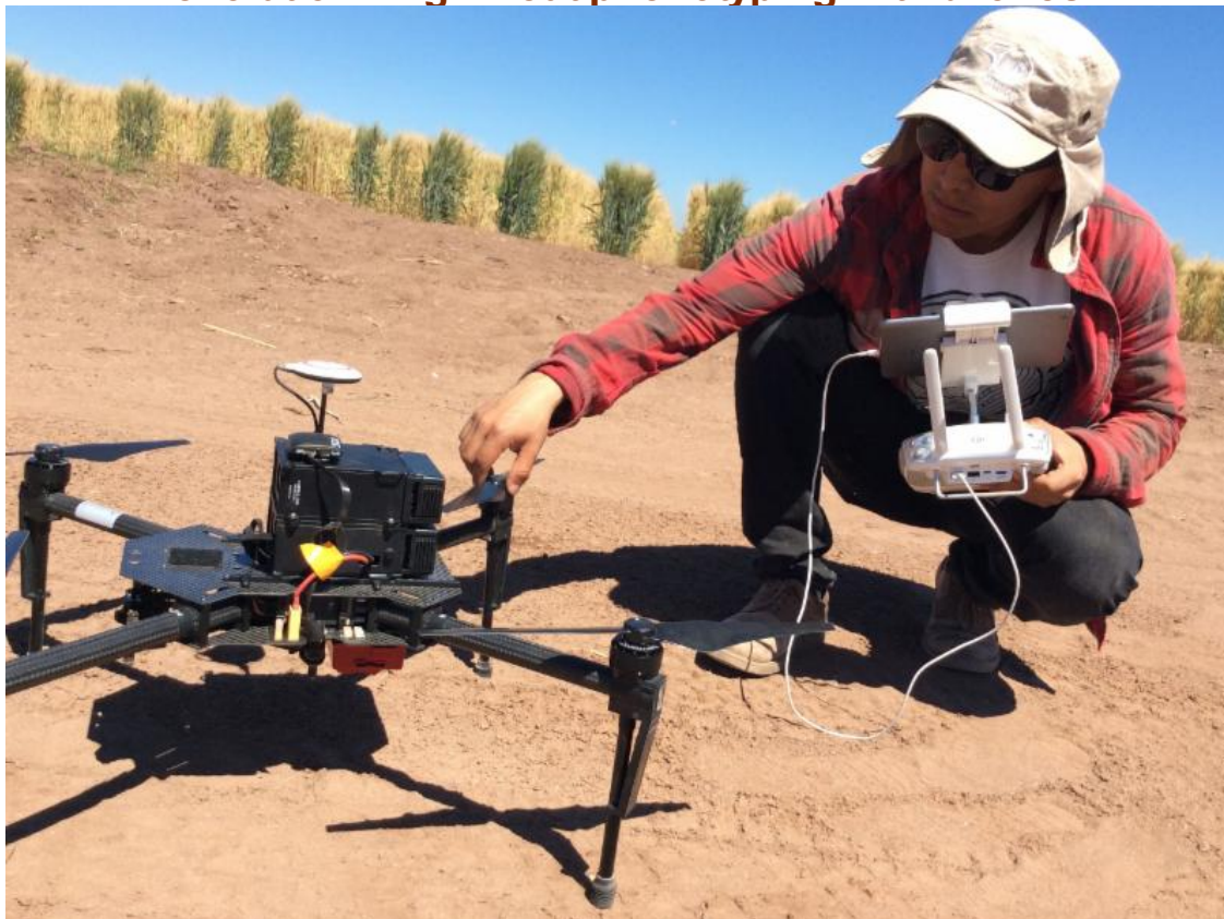
José Manuel Mendoza Reyes, with the physiology group at CIMMYT, calibrates a drone for small plot survey. This data could be used to enhance predictions about wheat line performance. Photo: Cally Arthur
